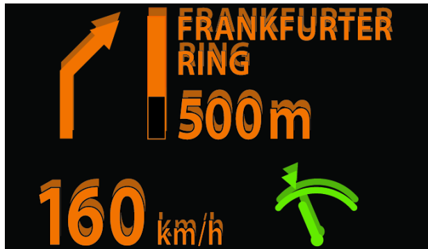
HUD image showing "double image" from incorrect windshield or incorrect windshield installation
